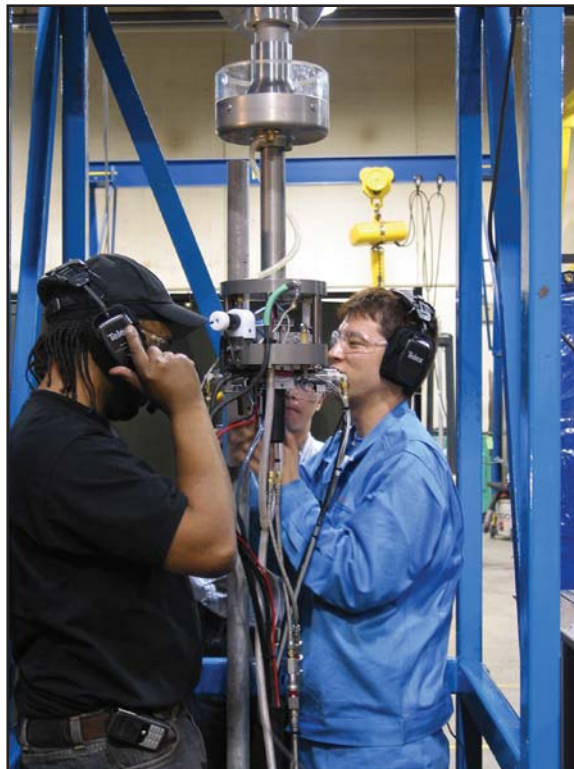
Thermal Sleeve Cutter in Mock-Up
